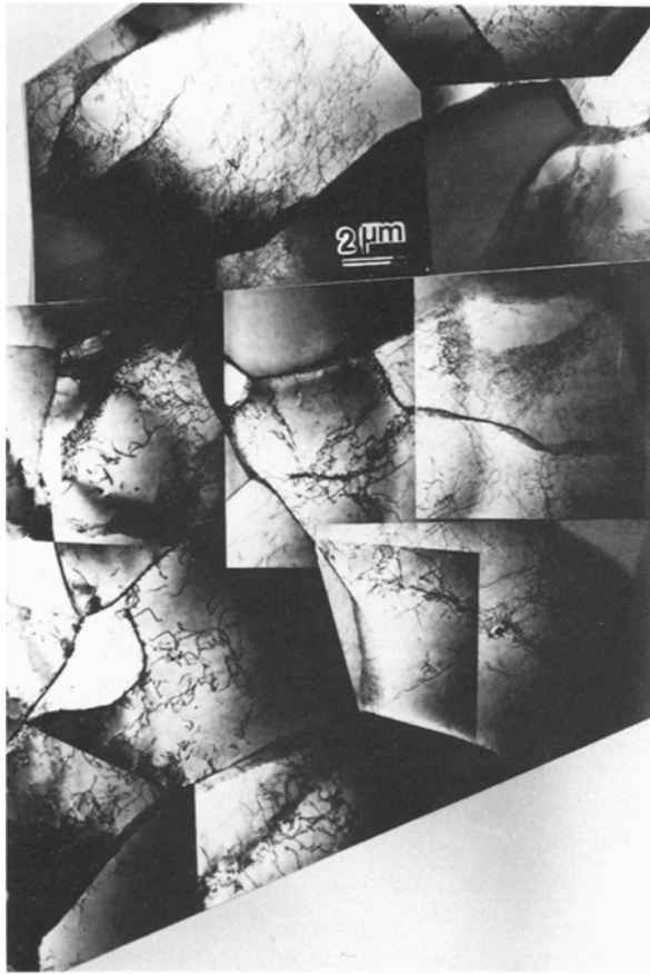
Figure 5 Typical subgrain structure in the neck ( \epsilon = 51\% ). One subgrain (bottom right) is subdivided into smaller subgrains.
